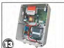
13 DC Converter Provides battery backup to the system
